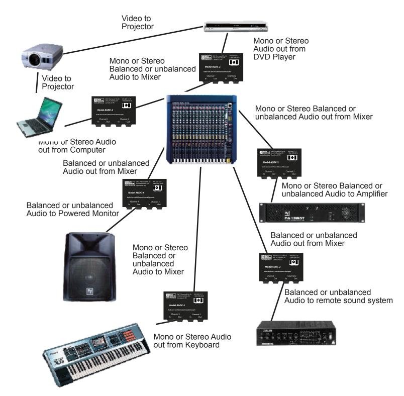
NOTE: All inputs and outputs are Line level, not Microphone level.
