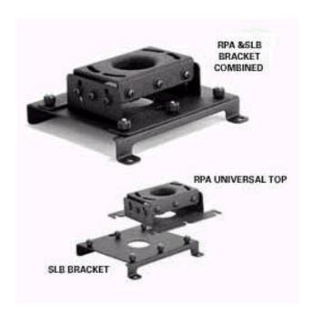
Chief's RPA Series Ceiling Mounts provide a uniquely simplified method of mounting an inverted LCD projector to the ceiling. Each RPA ceiling mount consists of a basic ceiling mount housing with roll, pitch and yaw adjustments and a projector hanging bracket specifically designed for each LCD projector. This custom designed bracket provides convenient lamp, lens and filter access as well as quick-release projector disconnect.
