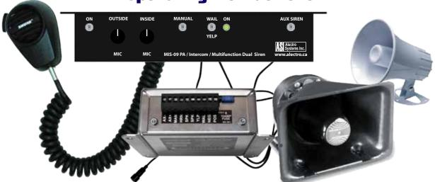
The MIS-09 was designed for the armored car and truck industry as well as Emergency Vehicles to allow the driver to communicate with a person outside, without opening a window. As well as an intercom, the MIS-09 also includes a Public Address System and a Full Function Siren which meets North American Emergency Vehicle standards.
