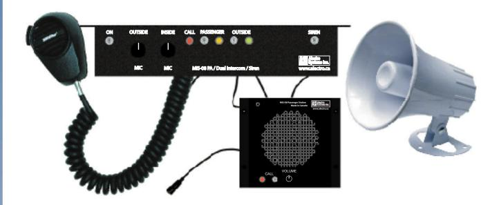
**Passenger Mode:** Press the "PASSENGER" button to set the system to passenger mode. This will illuminate the Amber light on the Main Unit. Adjust the Left Hand volume control (Outside), if required, to obtain the desired volume from the passenger microphone. You will hear this through a speaker built into the main unit.
