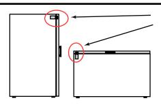
The DA-9ADP needs to be installed on the edge of the freezer or fridge **where the door opens, not the hinge side**. Usually the best place is on the side at the top.
