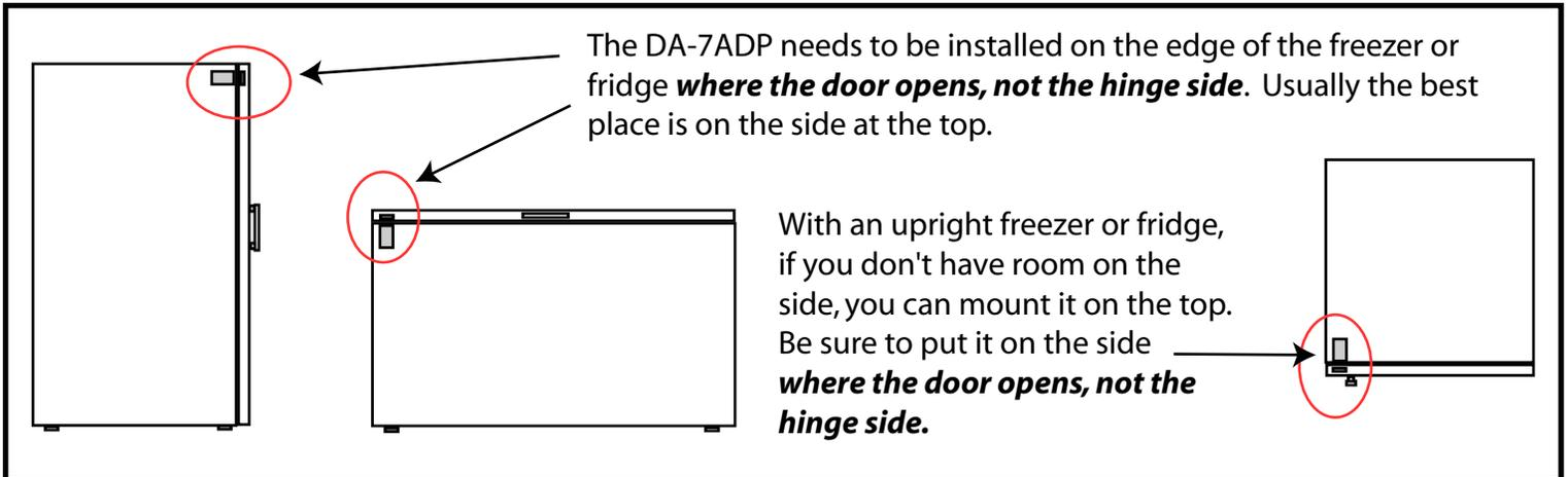
**STEP 1:** Once you decide where you will mount the DA-7ADP, clean the surface of the door and side of the freezer or fridge where the unit will be located. Make sure the surfaces are clean and dry before proceeding to step 2.
