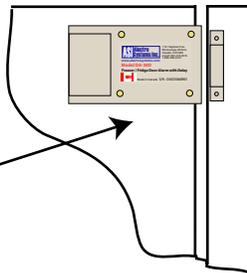
**Battery Replacement:** Open the battery cover, remove the old battery and replace it with a fresh 9 volt Alkaline battery. Place the battery inside the unit then replace the cover.
