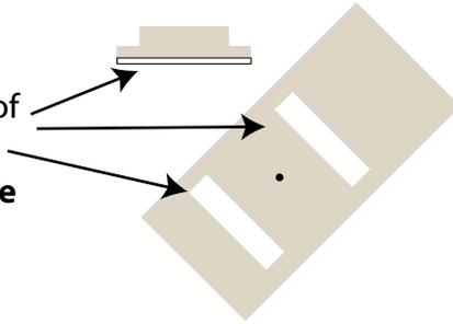
**STEP 3:** Carefully stick the Magnet on the Door of the freezer or fridge **as close to the inside edge of the door as possible**. Keep in mind that the DA-7ADP main unit needs to be located close to the magnet.
